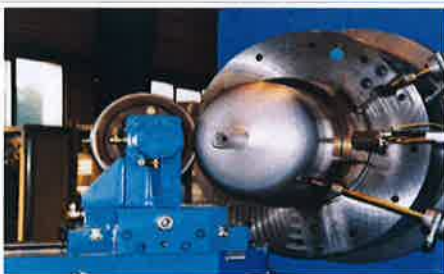
Process for hot forming and closure of cut-to-size tubes for pressurized gas cylinders.
