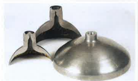
Process for hot forming and closure of cut-to-size tubes for pressurized gas cylinders.
