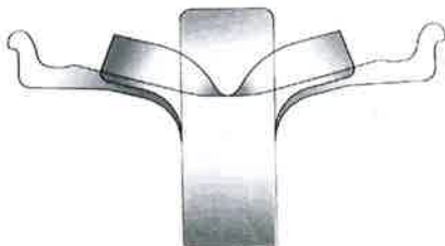
Process for the manufacture of aluminium wheels.
