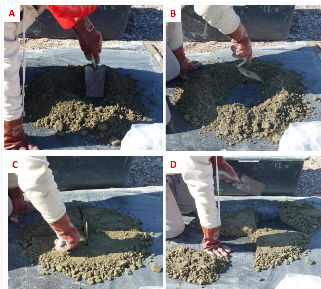
Figure 7-4: Core sampling method A) Sample flattened using corkscrew method; B) A ring is made; C) Sample is flattened and cut into quarters
