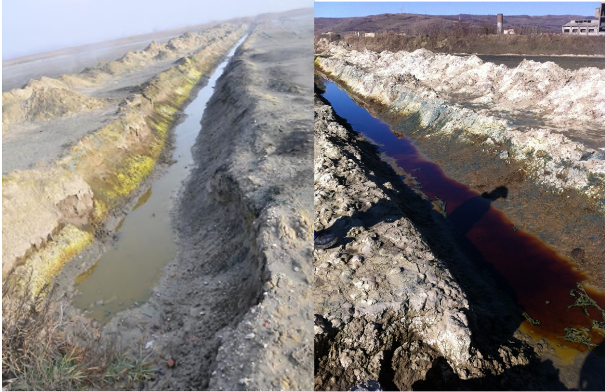
Figure 3: Chromium salt enriched drainage channel in Cell 4. Note the chromium salts retained by the clay alluviums along the length of the channel.
