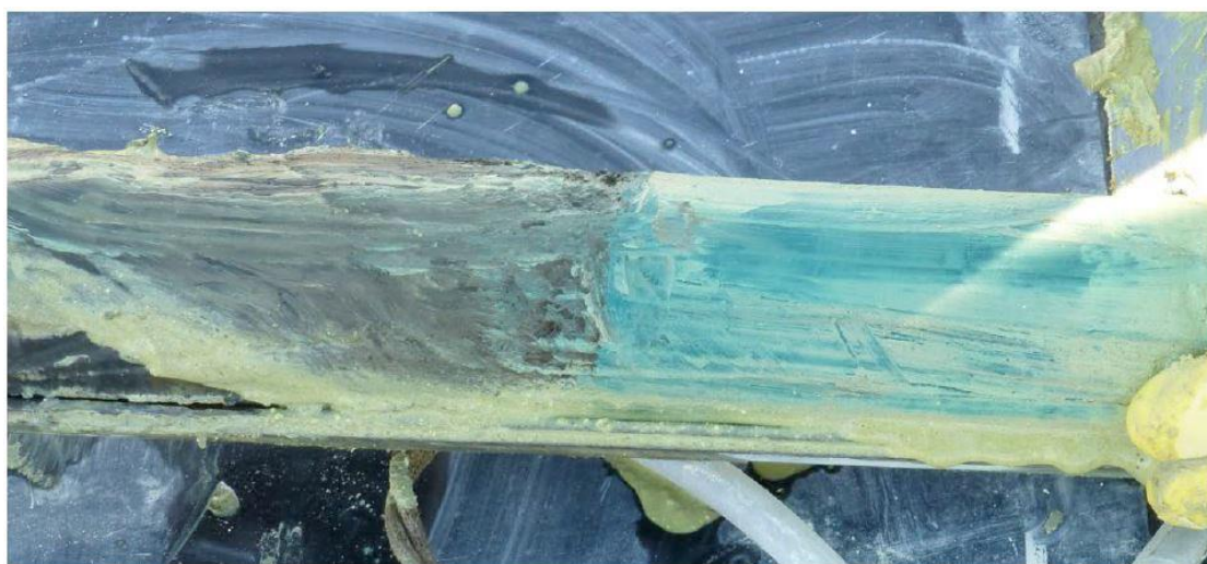
Figure 13-2: Base of the WSF, with the transition from green COPR on the right to the clay layer on the left
