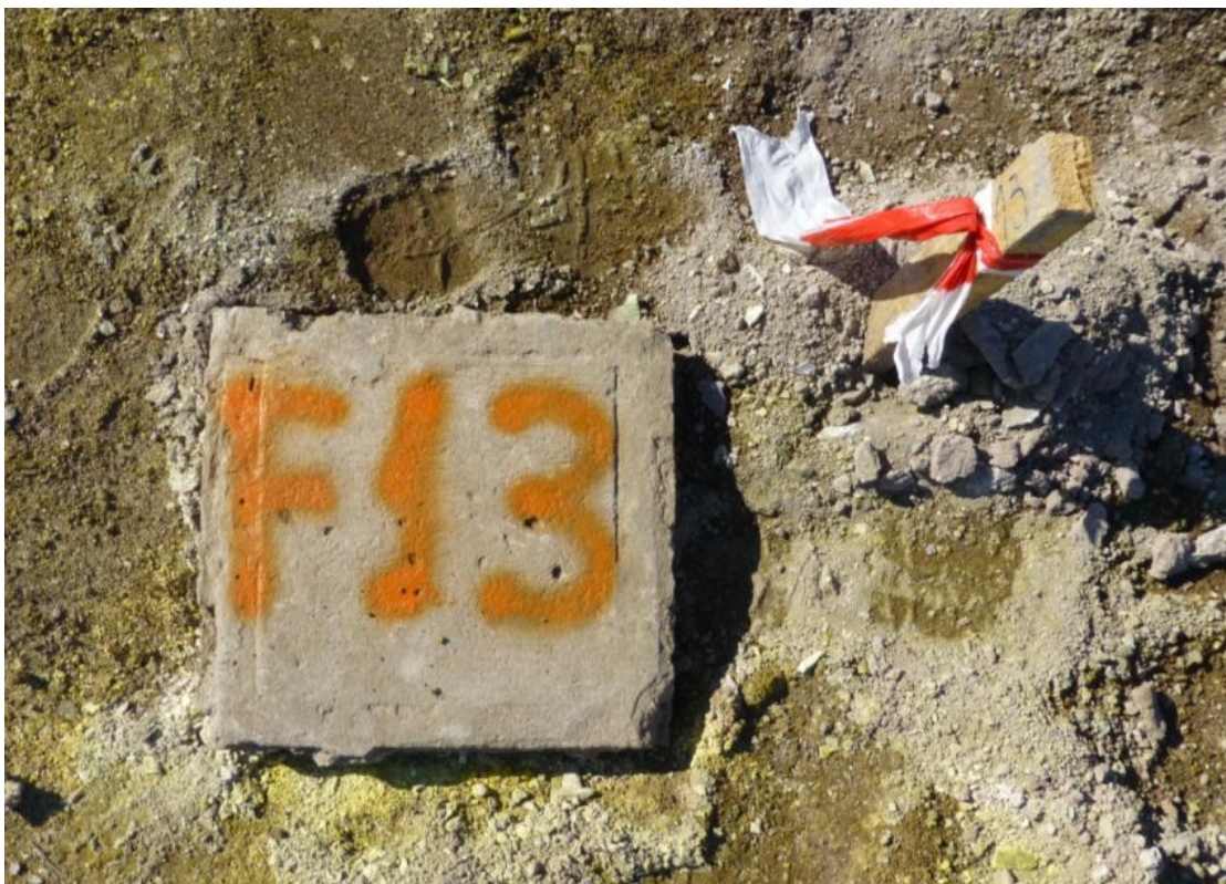
Figure 7-3: Completed drill hole collar marked and labelled
