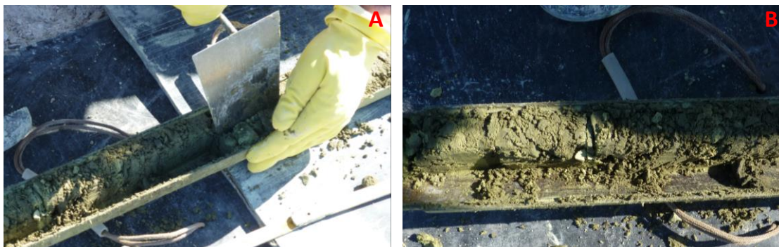
Figure 7-5: Auger sampling method, A) Half core sampling; B) Half core sample
